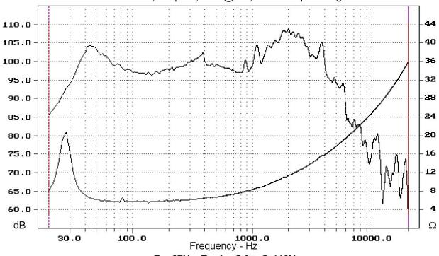
Fs: 27Hz, Z-min: 5.9Ω @ 110Hz
