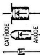
types are electrically equivalent. Connect the CATHODE lead of one of the rectifier diodes to lug #1 (curved line symbol) of the filter capacitor. Connect the ANODE lead to lug #2 of the 5-lug terminal strip (S). IMPORTANT: Arrange the diode leads exactly as shown in the pictorial diagram. When soldering,
