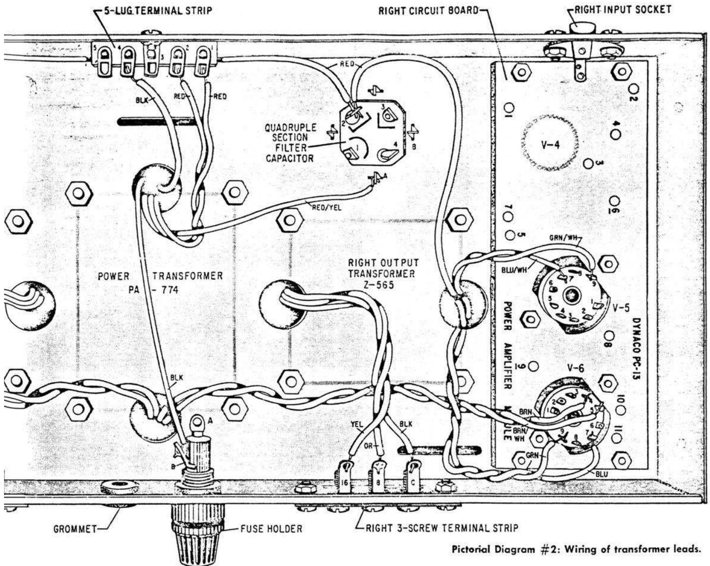
Pictorial Diagram #2: Wiring of transformer leads.
