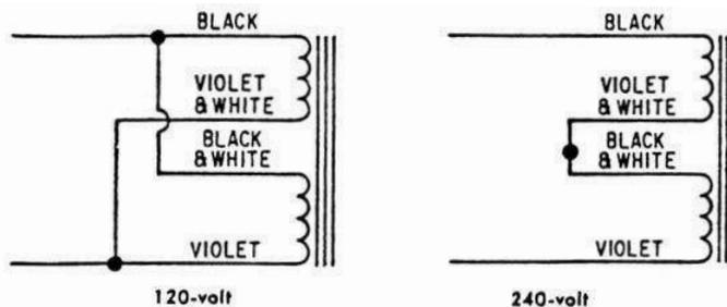
Dynakit Stereo 35 amplifiers supplied with power transformer PB-028 can be wired for used with either 120- or 240-volt a.c. power sources, in the following way:
