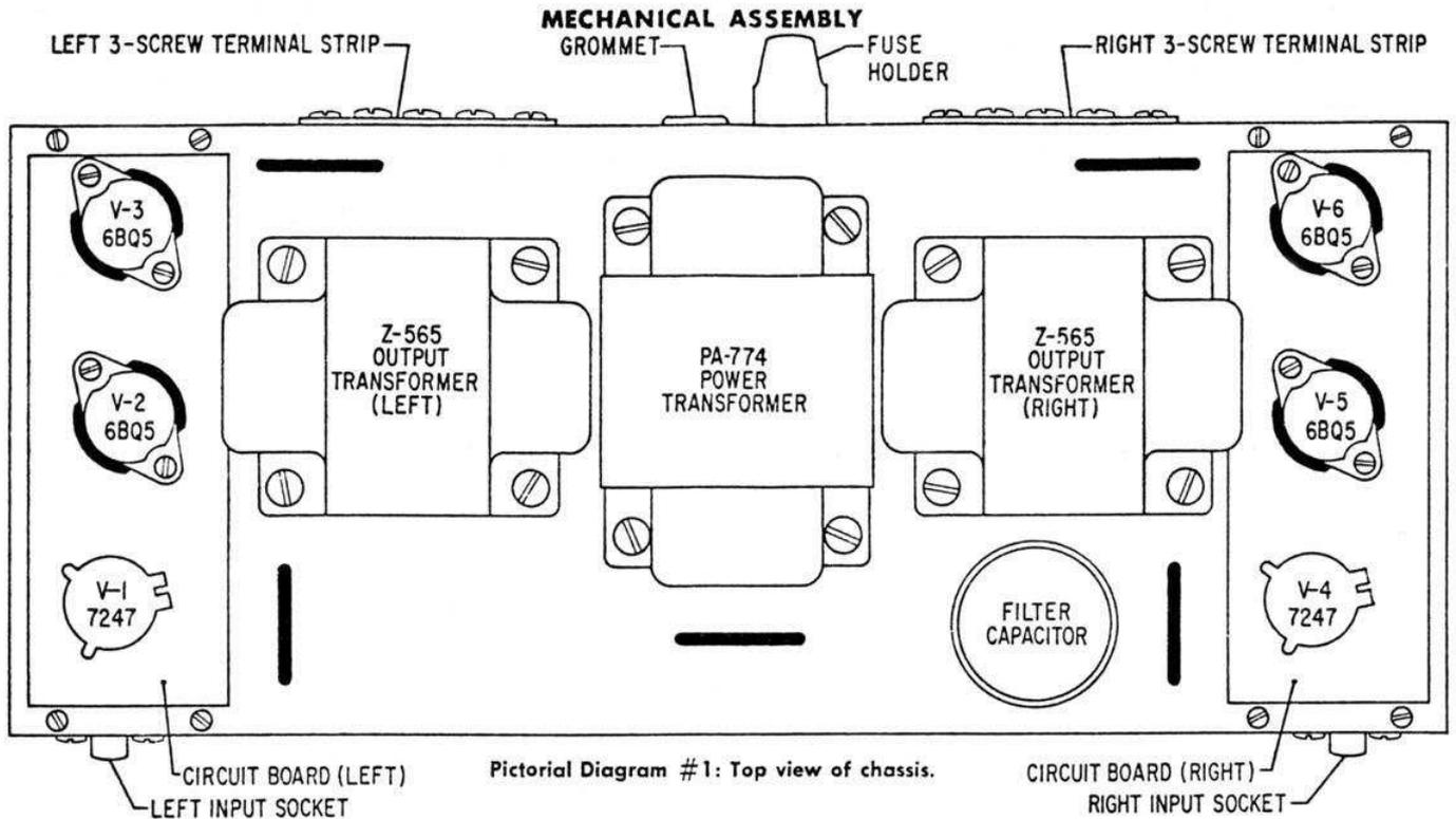
Pictorial Diagram #1: Top view of chassis.
