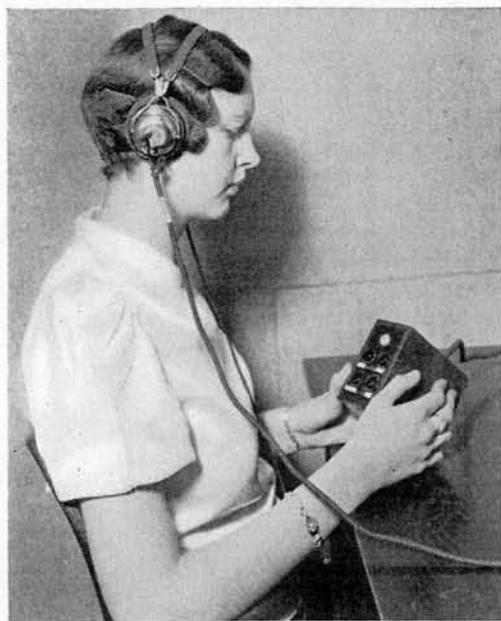
The apparatus at the right automatically presents a sound to be measured and a thousand-cycle comparison tone; the observer, Miss F. Torpadie, records her judgment as to which of the two sounds is the louder
